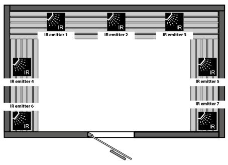
The IR emitters in this example have different tasks and should be con-trolled together in so-called channel groups.
