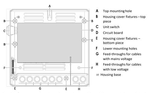
The cables for mains supply and low voltage can be routed through the existing holes on the back side or base of the housing.
