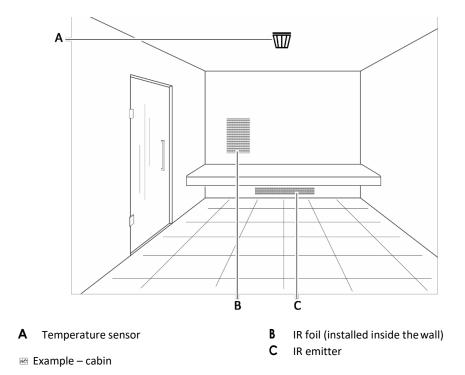
The position and number of IR emitters and foils (IR emitters) can vary depending on the design of the cabin.
