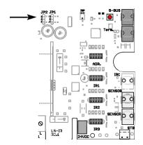
**2** Set jumpers JP1 and JP2 to foil (F) or emitter (R) depending on the connected emitters. See Emitter type – jumper JP1 and JP2.
