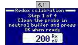
6.11 Example of first step of calibration with buffers. Continue with the following steps.
