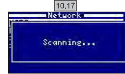
10.17 Select the desired network that the WIFI module can access. Enter the password in the pop-up keyboard. Scroll up and down with the up/down keys and left to right with the plus/minus keys. To select a letter press OK.
