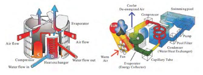
Heat pumps use heat from the sun by collecting and absorbing energy from the outside air. This energy is then compressed and transferred to the pool water. Your existing water pump circulates the water through the heat pump, which is normally installed next to the pool filtration system, and the water warms up. The heat pump timer can be set so that the pump operates at the times you want: for example, during daylight hours from 9am to 5pm.
