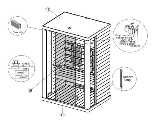
Note: connect all cables on the roof of the cabin
